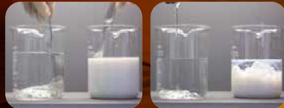
Self-emulsification of Easaqua™ Shows hand mixing of Easaqua™ (right) and standard hydrophobic isocyanate (left)
